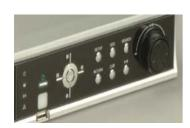
The various buttons on the front panel provide easy control of most DVR operations, such as camera selection, screen mode selection, search and pan-tilt-zoom control.
